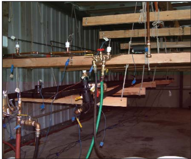
Figure 3. Test Rig for Uninsulated (Top) and Insulated (Bottom) Copper Piping
